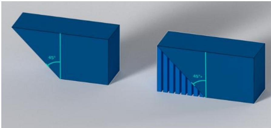
**Left:** If the overhang is 45° or less taken from the vertical, support are generally not needed
