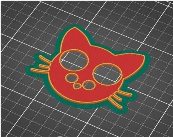
The **brim** serves to *increase adhesion to the bed, reducing the risk of warping*. A wider first layer is printed around the model. This makes sense especially if the model only touches the bed in a small area. This function can be enabled in PrusaSlicer by checking the "Brim" box in the menu in the right column. After the printing is finished, the brim can usually be removed easily by hand, or you can use a knife or scalpel.
