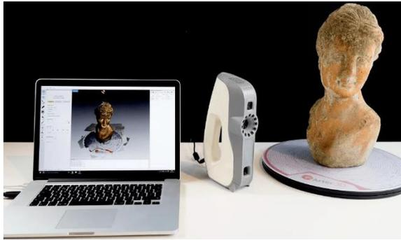
**3Dscanning** or *active sensing* is used to *collect data* about the form and structure of existing objects. The sensing system generates light or laser and uses a camera to capture generated pattern on real object.
